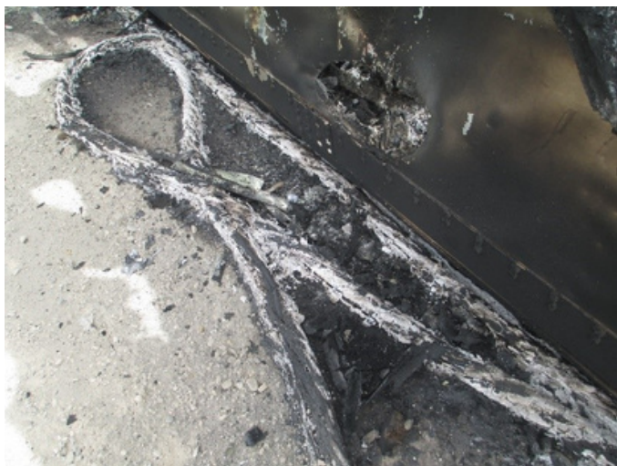
A mobile facility cable caught fire in OEF, resulting in facility destruction. Photos by Gunnery Sgt. Michael D. Sweeney
