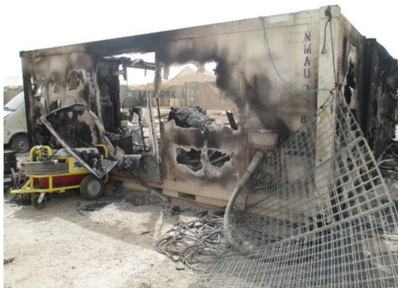
A mobile facility cable caught fire in OEF, resulting in facility destruction. Photos by Gunnery Sgt. Michael D. Sweeney
