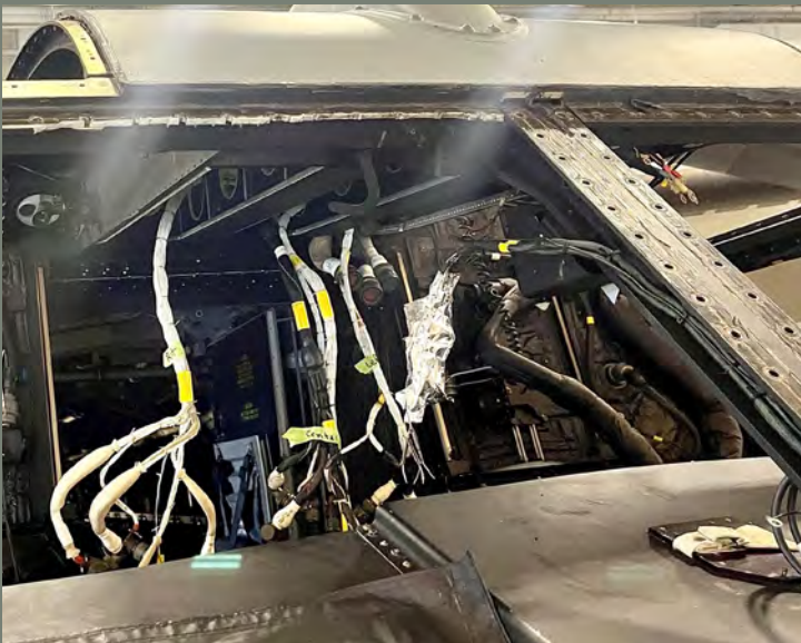
Aircraft ready for structural repair. Note the top shear line through the screw holes where the support structure failed.
