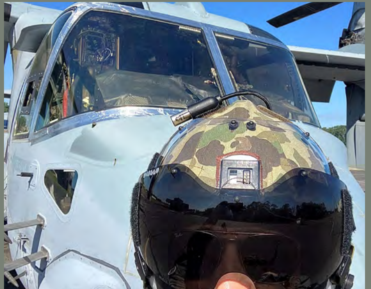
Aircraft after the windshield was replaced for one-time flight back to base. Note the heavy use of speed tape.
