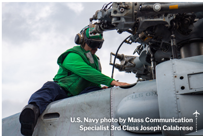
U.S. Navy photo by Mass Communication Specialist 3rd Class Joseph Calabrese Aviation Structural Mechanic (Safety Equipment) 3rd Class Austin Whitehead performs maintenance on the rotor head of an MH-60R Seahawk helicopter.
