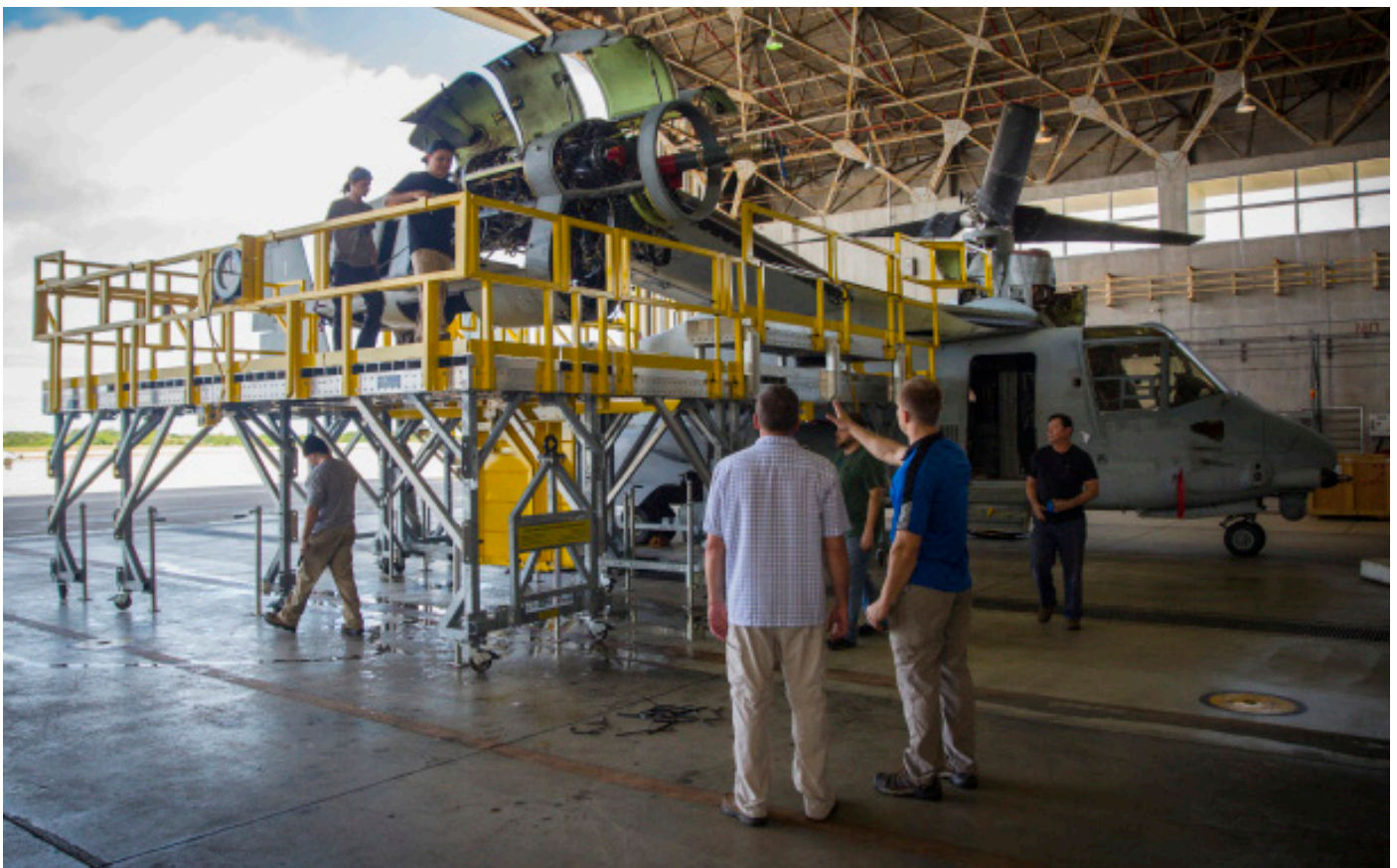
Aircraft maintenance contractors use a FlexDecks Osprey Wing and Nose Stand to maintain an MV-22B Osprey at Marine Corps Air Station Futenma, Okinawa, Japan. The platforms offer full nose and wing fall protection and enhanced worker safety while creating a more proficient maintenance process. (U.S. Marine Corps photo by Cpl. Andy Martinez)
