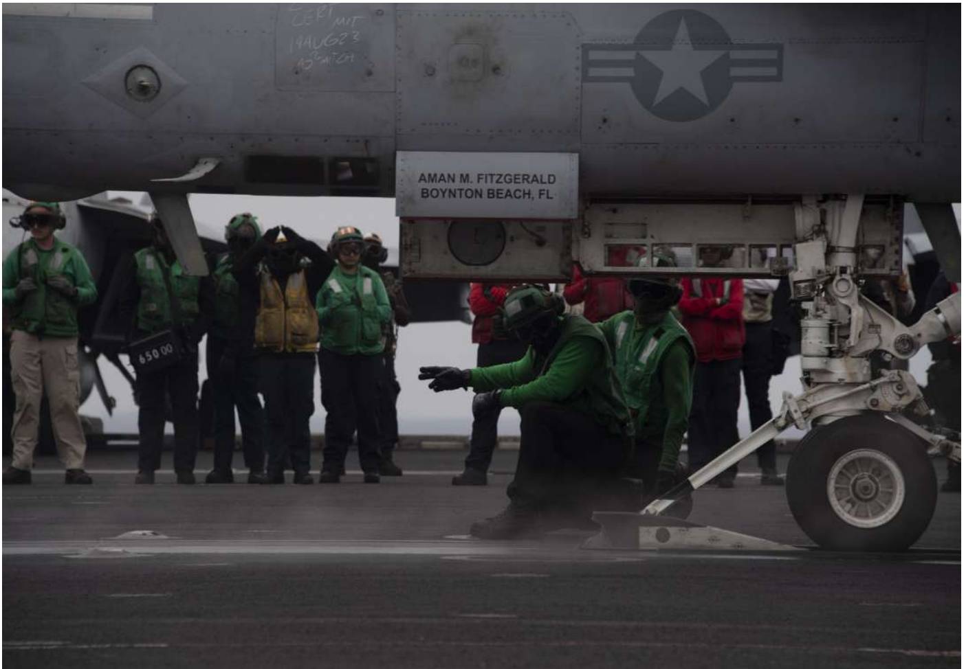
Sailors guide an F/A-18F Super Hornet, assigned to the "Bounty Hunters" of Strike Fighter Squadron (VFA) 2, into a catapult shuttle on the flight deck of Nimitz-class aircraft carrier USS Carl Vinson (CVN 70), Aug. 25, 2023. (U.S. Navy photo by Mass Communication Specialist 3rd Class Larissa T. Dougherty)
