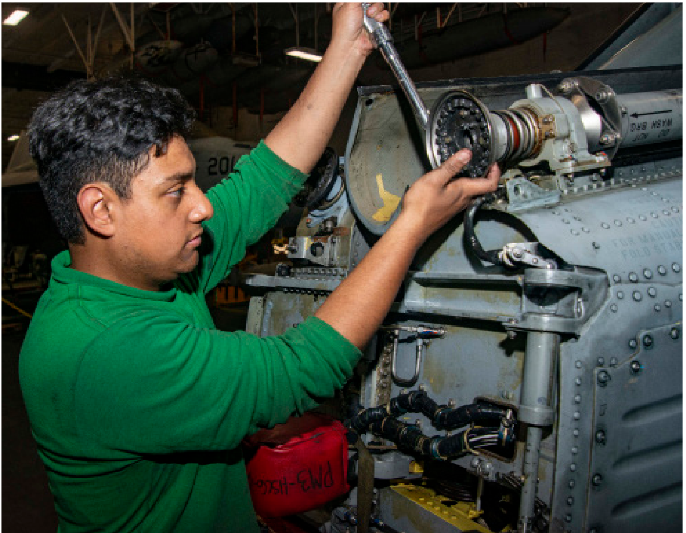
U.S. Navy Aviation Machinist's Mate 3rd Class Anthony Avilatorques the flex-coupling of an MH-60S Sea Hawk helicopter in the hangar bay aboard the aircraft carrier USS Nimitz (CVN 68) April 5, 2023. (U.S. Navy photo by Mass Communication Specialist 3rd Class Caylen McCutcheon)
