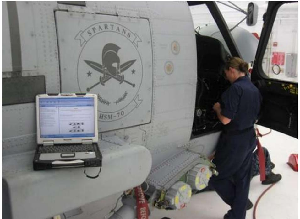
A PEMA in use during MH-60R maintenance at HSM-70. Photo courtesy of NAVAIR.
