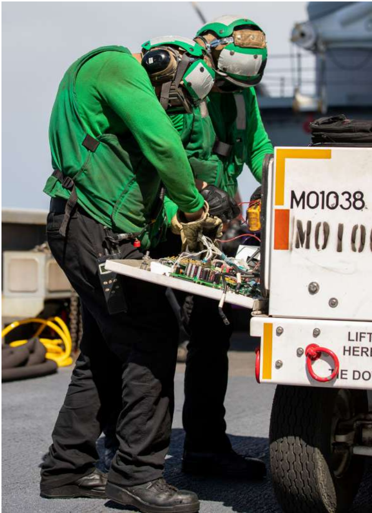
Aviation Support Equipment Technician 2nd Class Issac Contreas, and Aviation Support Equipment Technician 2nd Class Juan Vaulkens, both assigned to USS Gerald R. Ford's (CVN 78) aircraft intermediate maintenance department, perform routine maintenance on a static frequency converter, Oct. 11, 2022. (U.S. Navy photo by Mass Communication Specialist 3rd Class Grant Gorzocoski)
