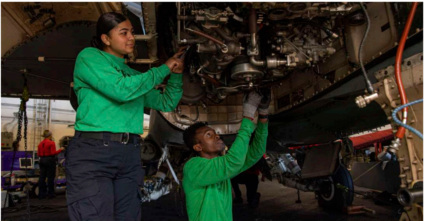
Aviation Machinist's Mate 2nd Class Ashley Miranda, left, and Aviation Machinist's Mate Airman Jan Michael Simmonds, remove an engine from an F/A-18F Super Hornet from Strike Fighter Squadron (VFA) 22 aboard USS Nimitz (CVN 68), Aug. 23, 2023. (U.S. Navy photo by Mass Communication Specialist Seaman Tomas Valdes)
