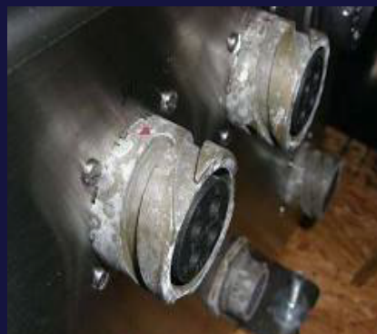
Cadmium Bloom corrosion on connectors and fasteners
