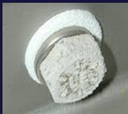
Cadmium Bloom corrosion on connectors and fasteners
