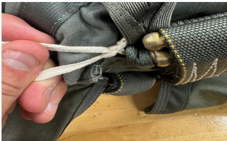
Figure 1 - Locking knot on riser connector
