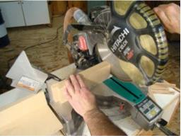
Another hazardous tool you might have in the shop is a miter or chop saw (pretty simple - one is able to chop and miter, while the others can't). The miter saw is a valuable wood cutting tool allowing one to make angled bevel, miter cuts or right angle cuts and is the most efficient tool for jointing. This tool seldom leads to serious injury, except for the ten unlucky Sailors and Ma-
