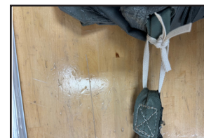
Knot on Canopy Deployment Bag, (left)
