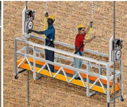
Two Point Scaffold
