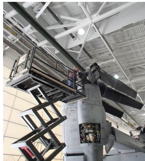
Mobile Man lift (MML) provides tremendous utility as platform has telescopic extension
