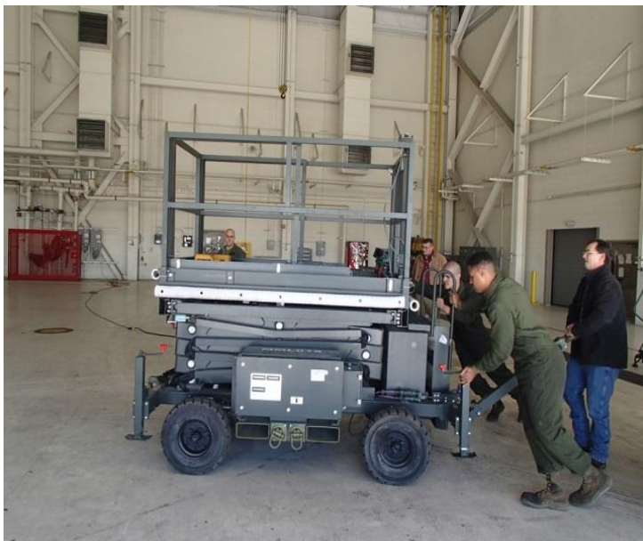
Mobile Man lift (MML) in non-powered and is authorized a peculiar SE for MV-22 and E-2D
