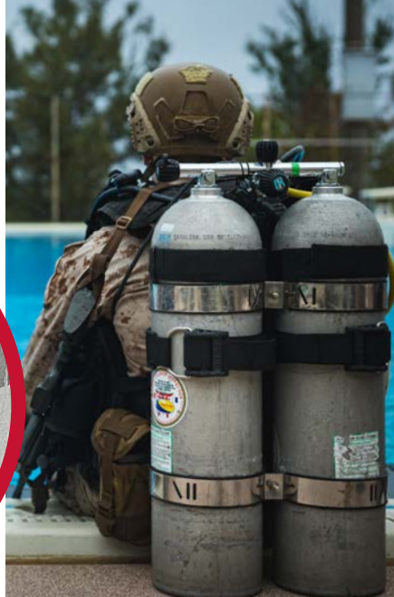
Figure 2: Aqualung twin cylinder adapter kit P/N 18252. Marines in training on Camp Schwab, Okinawa, Japan, Feb. 8, 2024. (U.S. Marine Corps photo by Lance Cpl. Matthew Morales)
