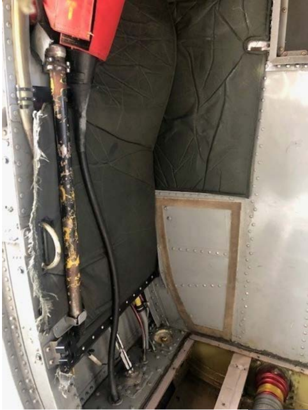
AUX tank APU pump handle position U.S. Navy photo by Senior Chief Naval Aircrewman Wade Hove
